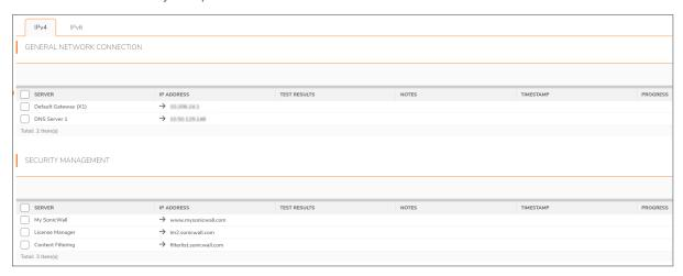
This tool helps you locate the problem area when users encounter a network problem. The feature lists both IPv4 and IPv6 network settings in different tabs.
