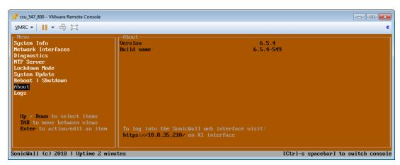
8 Switch consoles to verify that SonicOS is updated to the new version, and that the NSv is still registered and X0 still has the configured IP address.
